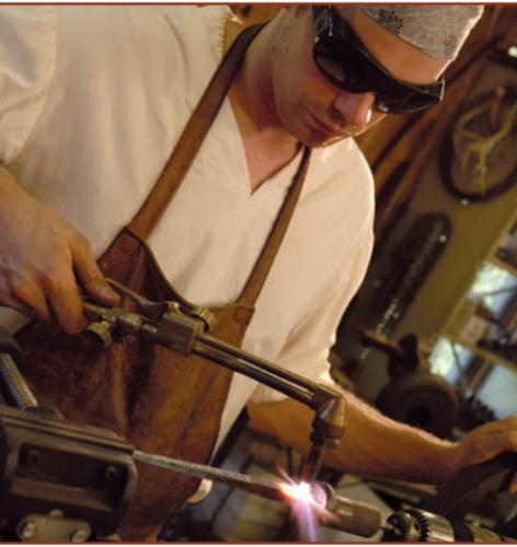
Daniel, twisting a piece of 1/2" tapered steel using the modified drill press described in the article.
